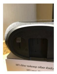
**Step 1** of Set Up: Pull the plastic tab on the bottom which will engage the lithium ion battery for back up.
