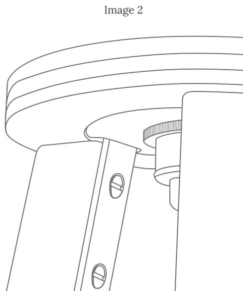
Before attaching your lampshade and lamp holder to the stand, you first need to attach the legs of the tripod to the plywood top plate.
