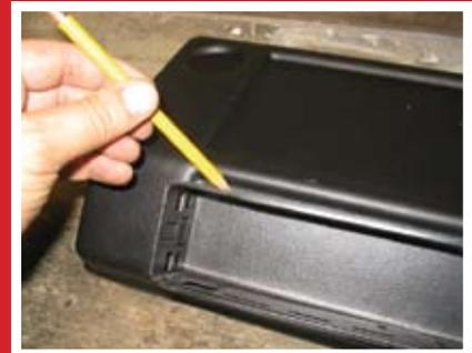
To relocate the cigarette lighter you'll need to drill a 28mm hole in the console. The socket can be positioned in either of the recessed circular mouldings. On Soft-Top and Pick-Up models, the vacant recess that would normally house the rear wiper switch provides you with the option to fit another cigarette lighter socket to use as secondary 12v power supply. If fitting one of the MUD marine grade 12v sockets you'll need to drill a 30mm hole.
