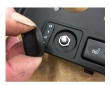
The clock is held in place with 4 x TX15 screws Using a magnetic scrwdriver makes their removal and refitment easier. With the clock removed, release the securing tab on the hazard switch with a thin bladed screwdriver.
