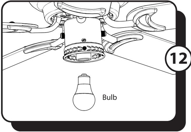
12. Install the E26-base LED bulb in the socket.
