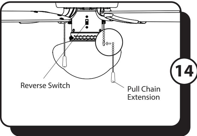
14. Attach the pull chain extensions to the fan and light pull chains.
