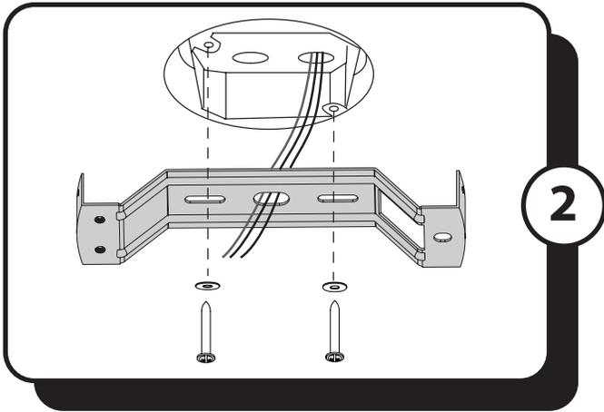
2. Secure the upper mounting bracket to the outlet box using screws, spring washers, provided with the outlet box (not included).
