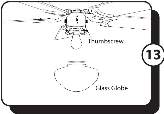
13. Loosen the three thumbscrews near the bottom of the light kit. Lift the glass globe into the light kit and retighten the previously loosened thumbscrews to secure.
