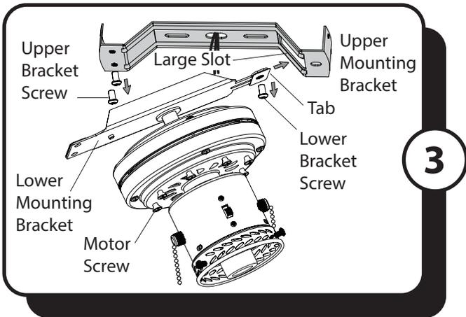
3. Remove the preassembled lower bracket screw from the lower mounting bracket and the upper bracket screws from the upper mounting bracket. Remove the motor screws and set aside for later. Place one tab of the lower bracket into a large slot in the upper mounting bracket.
