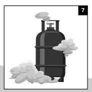
If there's a gas leak you cannot fix, do not use or move cylinder. Turn off the gas at the cylinder, disconnect the fuel line, and contact your gas supplier for repair. For severe leaks or fire, call the fire department.
