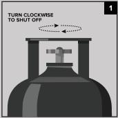
Ensure the cylinder valve is fully off.
