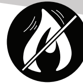
NOISY FLAME (EXCESSIVE OXYGEN)
