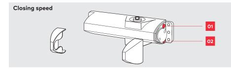
The closing speed of the TS 90 Impulse is adjustable in two independent ranges at the valves indicated.
