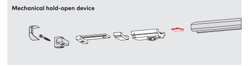
The hold-open device enables doors to be precisely held without any fall-back up to an opening angle of approx. 145°. The hold-open device is suitable for both LH and RH doors and is designed for retrofitting to the slide channel. **Not for fire and smoke doors.**
