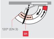
Cushioned limit stay for retrofitting by insertion in the slide channel. Adjustable between 80° and max. 120°. Use of the cushioned limit stay helps to prevent a normally opened door from colliding with adjacent walls. The cushioned limit stay is not an overload protection device and in many cases is no substitute for a door stop. Only for the use of TS 90 Impulse size EN 3.
