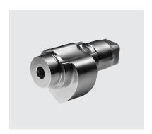
The heart-shaped cam and linear drive mechanism of the TS 97 ensure that the resistance encountered decreases almost instantly with the door opening action – so even children, the elderly and people with disabilities have no problem in passing through. User-friendly and reliable closing is also ensured by the delayed increase in the actuating torque at the 'latching' end of the sweep.
