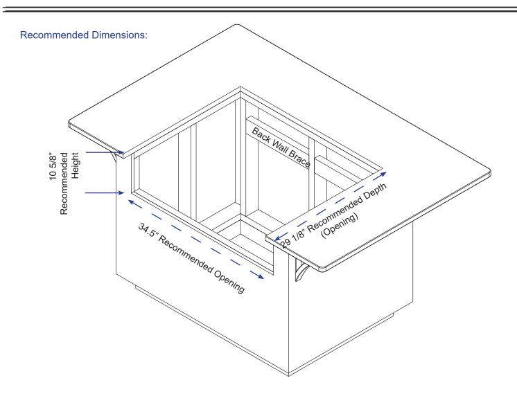
**STEP 1:** Prepare cabinet construction using either wood or steel framing. It is recommended to have a cutout measuring 29 1/8" depth by 34 1/5" width by 10 5/8" height.
