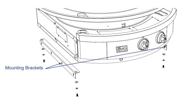
**STEP 6:** Remove two (2) mounting brackets with 7/16" Open End Box Wrench installed on Evo Affinity 25G Cooktop.
