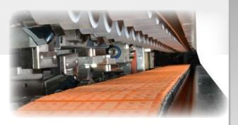
The presure bar, made from two rows of idle rubber rollers, is adjustable by a handwheel complete with a mechanical numerical indicator.
