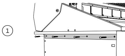
First you will need to remove the angle brackets from the side of the unit and replace them with cart mount brackets.
