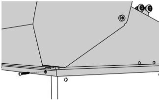
Secure the head to rear of cart with Phillips-head screws provided (10-24 x 1/2").
