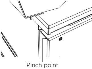
Position tabs on side bracket to fit into slots on the cart. When complete, the landing ledge should sit flush on the top of the cart.
