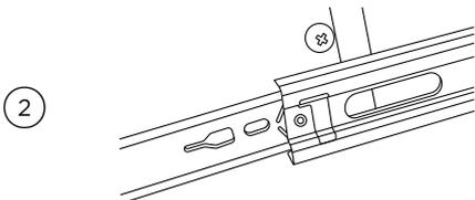
While holding the drawer parallel to the cabinet, carefully align & engage the ends of the glides. Slide the drawer about an inch so that the glides are supporting the back of the drawer.
