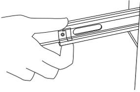
While holding the drawer up by the handle, pull the glides from the drawer cavity out over the drawer glide until they click.
