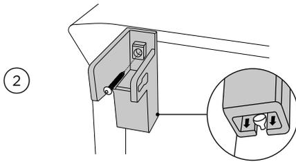
Slide left and right side shelf brackets over the shoulder bolt and install top screw attaching the side shelf brackets onto the cart. Tighten with Phillips screwdriver.
