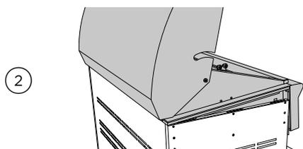
Placing head on cart, place rear of head over the rear of the cart first. Then allow the rear side tabs to first locate in the slots on the top of the cart sides. The other tabs will locate in the middle and front slots as the head is lowered into position on the cart.
