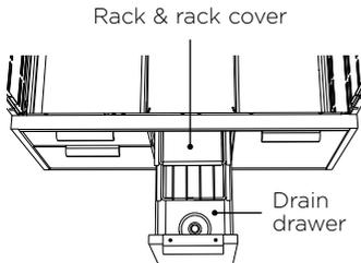
Install the two racks provided into the opening by sliding them onto the rollers on the sidewalls of the left cavity.
