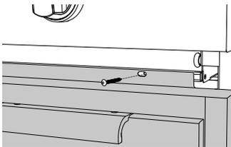
Install remaining screws (10-24 x 1/2") into the front of head to the cart.
