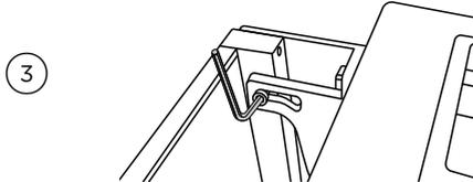
Holding the side shelf, install two shoulder bolts into the slot and screw into the side shelf tray. Tighten with a 3/16 Allen wrench.
