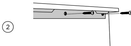
Install the bracket tab on both sides using eight of the 10-24 x 1/2" screws. Install each bracket with four screws on each side of the grill head. For a CAD1-48/48E, use the appropriately labeled bracket for your grill head and cart side.
