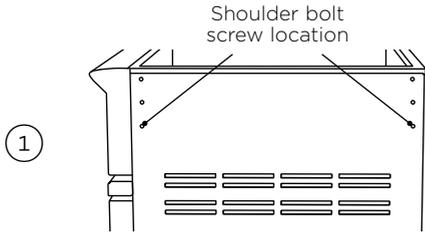
Screw two shoulder bolts into the bottom screws on the side of the cart. Tighten with 5/32 Allen wrench.
