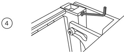
Place shelf in the up position and check for level. If shelf is not level, adjust side shelf set screw. Set screws can be adjusted using a 3/32 Allen wrench. Turn the Allen wrench clockwise to raise the shelf. Turn 1/4 turn and review to see if the shelf is level. The set screws in the left and right bracket should be adjusted equally to ensure the shelf sits level.
