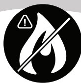
YELLOW FLAME (INSUFFICIENT AIR)
