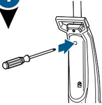
Insert screwdriver into the hole on the back of the unit below the Carry Handle in order to disconnect the handle.
