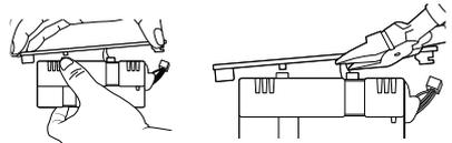
Pull the control panel back from the battery pack. Then, with rubber-handled wire cutters, clip the two metal poles to disconnect the battery pack from the control panel.
