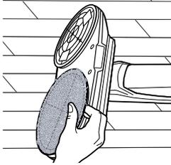
To remove mop pads, simply pull pads off the hook and loop material on the bottom of the machine.
