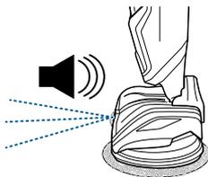
Formula will spray out of the nozzle on the front of the foot. You should hear a soft buzzing noise each time you press the SPRAY Button to indicate formula being dispensed.
