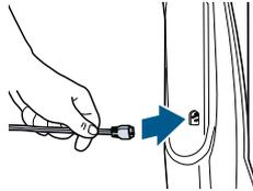
Insert the charging adapter plug into the charging port on the back, right side of the unit.
