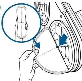
Then, with the mop pad folded, line up the small dot in the center of the pad with the middle screw on the bottom of the foot.
