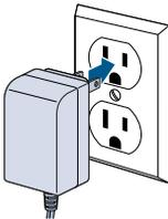
Plug the adapter into a suitable wall outlet. The battery status indicator lights will illuminate when charging.
