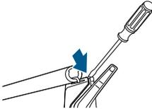
Insert flat-head screwdriver between the top front and back plates located between the Carry Handle and main handle to remove the front body plate.
