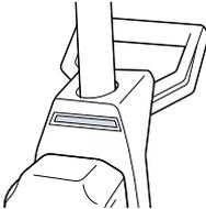
Before charging, make sure unit is OFF by ensuring the battery status indicator lights are not illuminated.
