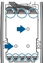
Disconnect the 8 inputs that are connected to the control panel. Then, using a Phillips-head screwdriver, unscrew the two screws on the control board.
