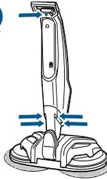
With a Phillips-head screwdriver, remove the 5 screws on the back of the unit.
