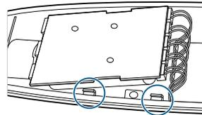
Remove the control panel with battery pack. For leverage, you may need to use the flat-head screwdriver to help remove.
