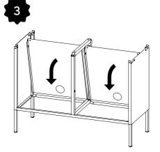
Push the back panels into place, starting at the bottom.
