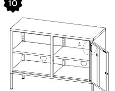
Slide the door down onto the post.
