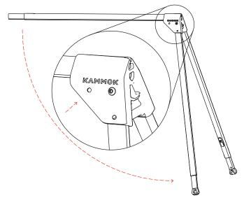
**3** Telescope the legs to the approximate desired height by pressing the top of the release lever.
