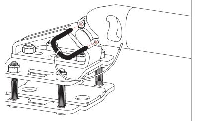
3 Loop the other included strap through the strap bar on the main pivot joint.
