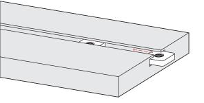
Position the ball hitch assembly over the T-slot nuts. Bolt securely in place using two of the hex head bolts.
