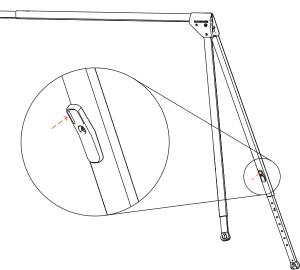
4 Attach the middle section of the structural ridgeline.
