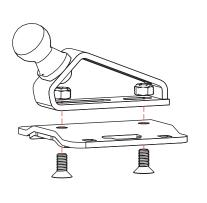
Insert the 4 longer hex head bolts through the bottom of the other clamp plate, and position the mount assembly on your rack/crossbars.
