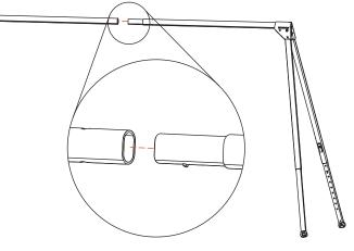
5 Attach the ball receiver section of the structural ridgeline.
