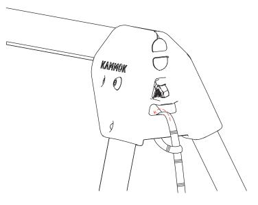
2 Loop the one of the included straps through the hole on the hitch receiver.
