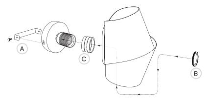
Only qualified persons should assemble the luminaire. If in doubt, consult a suitably qualified electrician. Installation MUST be carried out in accordance and compliance with current building regulations. This fitting must be earthed.
