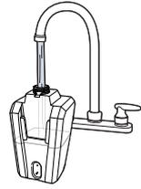
**3.** Fill with warm (140°F/60°C MAX) tap water to the WATER line. **Do not use boiling water. Do not heat water and/or tank in the microwave.**
