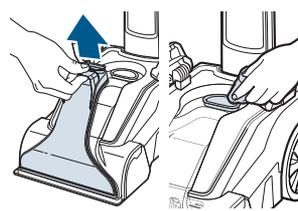
**2.** Grab the top of the Nozzle and pull it up and away from the machine. Rinse or wipe it clean. Use a cloth to wipe debris from the red filter.
