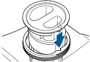
**6.** Once clean, assemble by aligning the arrow on the float with the notch on the tank. Then, return the ring and twist to lock. Make sure it's fully aligned, so water doesn't leak.
