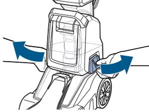
**2.** Release Dirty Water Tank by pulling out and up on the latches on the side.
