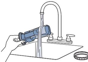
**5.** Clean and rinse debris from the float. Keeping the float clean prevents your Dirty Water Tank from overflowing and ensures the seal stays intact.
