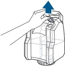
**4.** Lift tab on the top of the tank.
