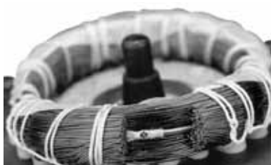
Fig. 48 PTC sensor incorporated in windings
