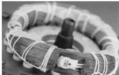
Fig. 50 Thermal switch incorporated in windings
