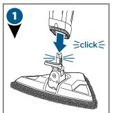
Attach lower body to mop head by snapping it into place.
