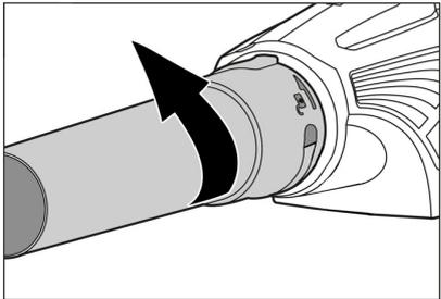
→ Turn the blower pipe in a counter-clockwise direction and remove it.
