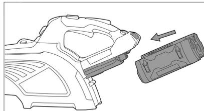
→ Push the battery into the retainer until it audibly snaps into place.
