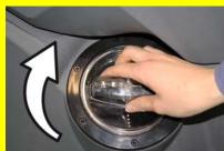
A Open the cover of the fresh water reservoir. Fill in fresh water (maximum 60 °C). Leave sufficient space for the detergent. Close the cover of the fresh water reservoir.
