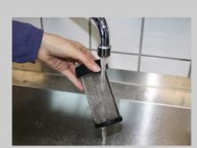
A Check and clean the waste water reservoir sieve.
