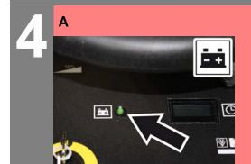
The battery indicator blinks A Charge battery.
