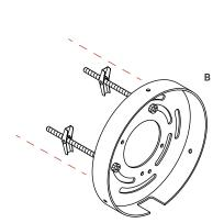
Step 2: Align the holes of the backplate (B) with the holes of the canopy cover (C). Secure them in place by twisting the thumbscrews (A) by hand.
