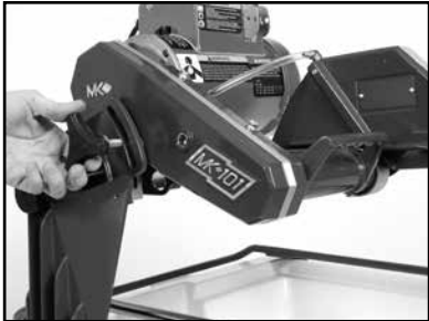
(A) Ensure the ON/OFF Switch is in the OFF position. Remove the blade and then Adjusting Knob.
