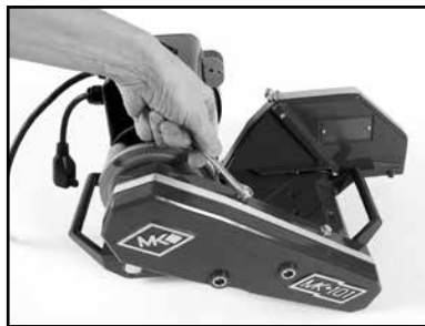
(Q) Install the Belt Guard.
