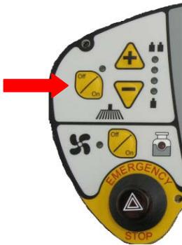
4. Press the "+" and "-" buttons to set the pressure of the brushes on the work surface.
