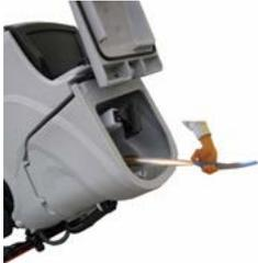
Check the suction filter is undamaged and clean.
