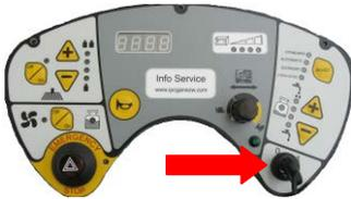
3. Press the brush button to enable brush and suction motor operation.
