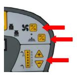
Choose the direction of movement by moving the direction selector. Select maximum speed by turning the potentiometer.
