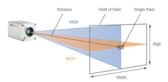
HFOV - Horizontal Field of View (horizontal aperture angle) VFOV - Vertical Field of View (vertical aperture angle)
