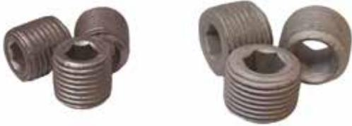
Spare Screws come in two sizes, 1/4" ISO 228 for the 20 and 25nb range and 3/8" ISO 228 for the 32, 40 and 50 ranges.
