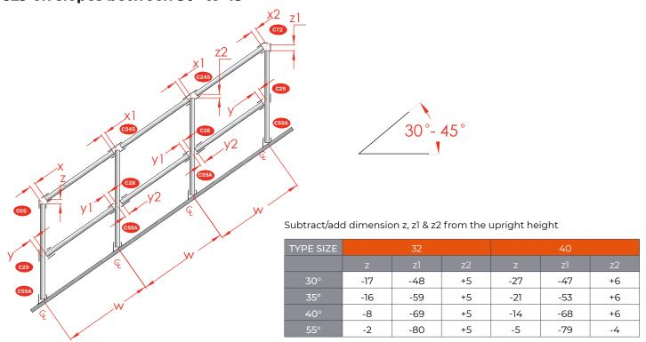
Subtract dimension x, x1,x2,y or y1 form upright centres (w). Please note the upright centres must be measured on the slope
