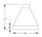
The Weather Cowl is designed to cover the Railing base and provides a weather proof seal when used with a suitable flexible sealant.
