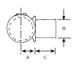
The Internal T joint is designed to provide an angled joint between a tube and a Flocon fitting when used in conjunction with CO2C and CO3C type fittings. Often used for railing tops and midrails to accommodate a slope as offset railing.
