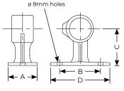
The Handrail Bracket is designed to secure handrail tube to a wall. It can also be used on top of walls as a fixing for a low rail.
