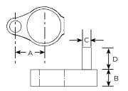
This fitting is designed as a gate hinge for light weight gates. If a heavy gate is being used we recommend that C03 and C30 type fittings are used to support the gate.
