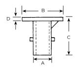
The Ground Socket is designed to provide a base that can be cast into the ground to support a post. The post is removable.
