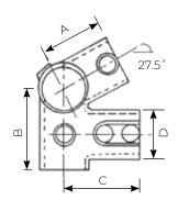
A four way socket fitting used to construct the eaves of a roof structure.
