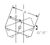
The Slope 2 Socket Cross is designed to provide a joint for the midrail for use on ramps. The variable angle allows the fitting to accommodate slopes up to 11°.
