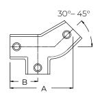
Used to form a Tee on handrails where the rail changes from level to sloping up the stairs. Adjustable between 30° & 45°
