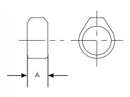
The Collar fitting can be used to support the CO3 fitting when the latter is used as a hinge. It can also be used to increase the load capacity of another fitting when used together.
