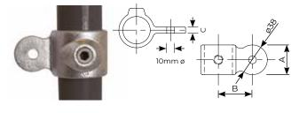
Can be used on its own for use with a shackle and chain or with the C36 female swivel to mount rails at any angle for slopes. It can also be used for attaching flat sheets or boards to a structure and is available assembled with the C36 fittings as a C45 single swivel combination.
