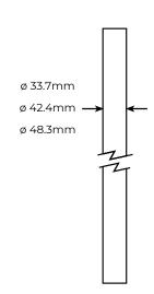
**Stair Return Bends** 33.7, 42.4 and 48.3mm handrail tube from stock
