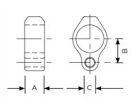
This fitting is designed as a gate eye for light weight gates. If a heavy gate is being used we recommend that C03 and C30 type fittings are used to support the gate.
