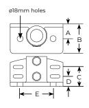
The Base Flange with Integrated Toeboard is ideal for guardrailing and balustrading applications where the addition of a toeboard is required. The side plates have slotted holes to allow for a degree of sideways movement for ease of installation.
