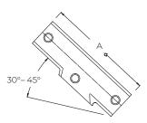
This fitting is used on Safety Railing with slopes between 30° & 45° and fixes the top rail to a vertical intermediate upright
