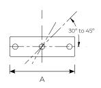
The Adjustable 2 Socket Cross fitting will accommodate any rake angle from 30° to 45°. This fitting is not recommended as the top fitting on a guardrail or balustrade system, use the C29 Adjustable Short Tee.
