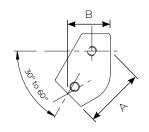
The Adjustable Short Tee fitting will accommodate any rake angle from 30° to 60°. This fitting is commonly used for the top rail of handrail to accommodate the rake angle on slopes. It can also be used for any Tee Joint to make at an angle of between 30° and 60° for light weight structures.
