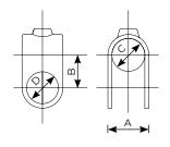
The Clamp on Crossover is designed to allow a new tube to be joined to an existing structure.
