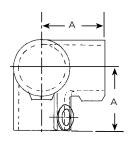
The 3 way 90° Elbow is designed to provide a neat corner for the upper rail of guardrail or frames.
