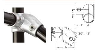
Used to form a Right hand Side Outlet Tee on hand-rails where the mid rail changes from level to sloping down the stairs. Adjustable between 30° & 45°
