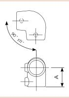
The Slope Elbow is designed to provide an elbow for use on ramps. The variable angle allows the fitting to accommodate slopes up to 11°.
