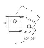
The adjustable Short Tee fitting will accommodate any rake angle from 11° to 30°. It can be used for any Tee Joint to make an angle of between 11° & 30°.
