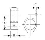
The fitting is designed to provide an attachment for flat sheets or board. It may also be used as a gate stop. An alternative fitting for the attachment of boards is the C35 type.
