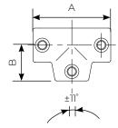
The Slope Long Tee is designed to provide a T joint between two tubes for use on ramps. The variable angle allows the fitting to accommodate slopes up to 11°.
