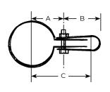
The Single Mesh Clip is designed to provide a fixing for standard mesh panels. It is recommended that the clips are spaced at a maximum of 450mm apart.
