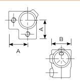
The Corner Complete with through tube is designed to provide a 90° corner for the intermediate rail of guardrail or frames.
