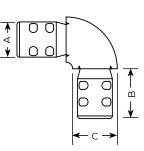
Crimp Elbow provides a permanent 90° connection for 33.7mm diameter x 3.2mm thick tube, a crimping tool is necessary.
