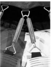
loading one side. Working in a circular motion around the tube, add 2 springs per side then go on to the next section and do the same. Eventually, you will have all springs attached.
