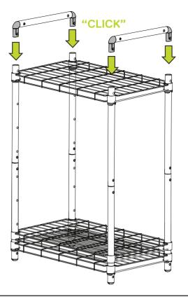
Determine the desired height of the middle shelf and then slide shelf above the selected holes. Attach the four plastic collars at the desired height.
