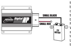
Optional: Programming of the Digital HP can be done before installing. This reguires a 9V battery. Attach the small black wire to the battery negative terminal. Program your settings. O When finished hold the small red wire on the battery positive terminal. The LEDs will blink indicating the setting is saved.
