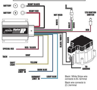
Do not connect Tach or B+ wire to distributor. Only attach the wires shown above to the distributor terminals.
