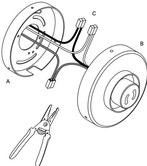
**Step 4:** Align the holes of the backplate (A) with the holes of the canopy cover (B). Secure them in place by twisting the thumbscrews (D) by hand.
