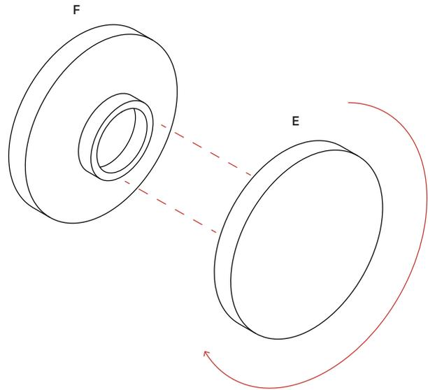
**Step 7:** Attach the shade assembly to surface mount by rotating clockwise until fixed in place. Turn the power back on at the main fuse box or circuit panel you disabled before installation.
