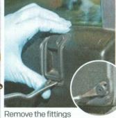
Pop the covers off the ends of the grab handle, undo the two screws and remove it. Undo the screw securing the interior door release and slide the surround away. Pop up the door lock trim, remove the window winder, and remove the two push-pin clips.
