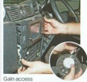
Next, there's a bit of dashboard stripping to do. Undo the two T30 Torx screws from the centre panel and unclip it, disconnecting the radio head unit, clock and switches as you go. Remove the driver's side speaker and open both of the fusebox panels.
