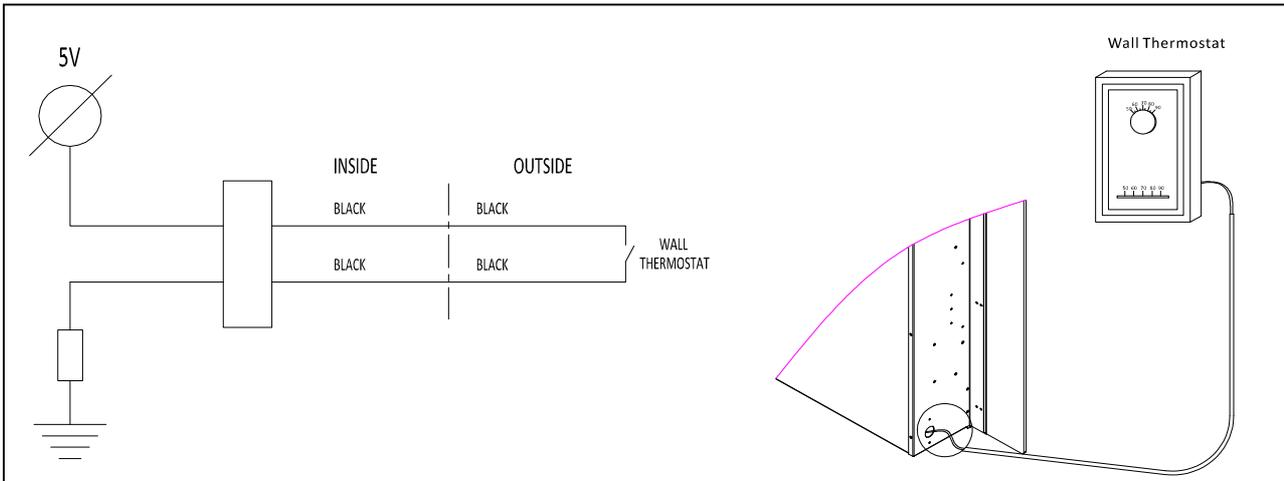
**NOTE: THE WALL THERMOSTAT WILL WORKING WHEN THE HEATER ON TEMP. SETTING. PLEASE REFER TO THE MANUAL CONTROL AND THE REMOTE CONTROL.**
