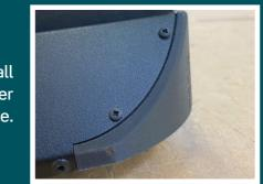
4. Use 4 x M6x16 fasteners and 4 x washers to install the 4 x Rubber Buffers to the backplate in the locations marked in the positions marked in the picture. Use a washer under the base of each rubber buffer. Tighten the buffer fastener with the T30 key while gripping the buffer between your fingers.
