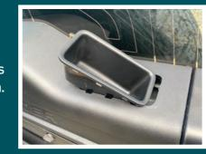
Use a trim-tool or pull firmly around the edge of the door-trim to release the trim clips from the door.
