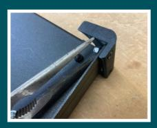
2. The upper corner trims are fixed using 2 x T10 x 8mm and 1 x T10x12mm fasteners and the M3 nyloc nuts. This is the fiddly part of the table install. Use the T10 screwdriver bit supplied on the fastener heads. If you don't have a spanner to hold the M3 nuts then a pair of needle nose pliers/grips can be used as an effective substitute.
