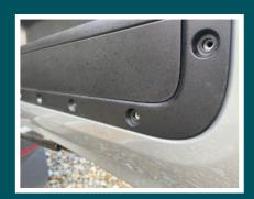
Remove the 11 visible Torx fixings on the rear door-trim using the T30 key supplied. You will not re-use these fasteners for the table install so store them away securely should you wish to remove the table in the future.
