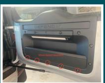
The longest sized spacer blocks (15mm) go across the five bottom fastener locations marked in RED.
