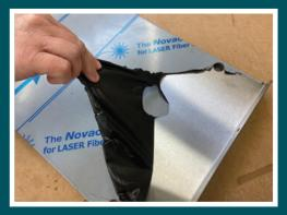
14. Peel off the protective film from the drop-down table panel. If removing the film reveals any printed text on the sheet metal, this can be removed by polishing with any acetone product.
