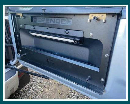
Once all of the fasteners have started in their threads and the spacers sit snug within their recess, tighten all 11 of the fasteners down. With the backplate installed on the door-trim you're now ready to install the fold-down table to the backplate.
