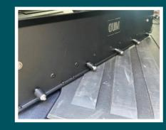
12. When you have all 11 fasteners and spacer blocks located and secured with anti-loss washers you're ready to attach the backplate to the door-trim.
