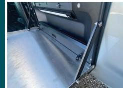
**16.** Use a pair of the thin plastic washers between the table support tabs and the slots in the backplate to prevent metal-tometal contact as the support tab slides in the channel. Tighten the nyloc nuts on the support tabs just enough that the tabs can still slide freely within the channel on the backplate.
