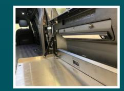
If you wish to fit a light to illuminate your table when in use then you WILL need to remove the door-trim from the door to install any wiring BEFORE fitting the table. We recommend using a spare/empty terminal within the vehicle fusebox to power your light.
