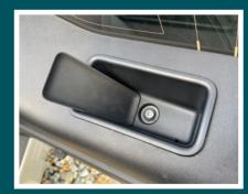
There is an additional hidden fixing within the recessed door-pull. Remove the rubber infill pad from the bottom of the door-pull recess to reveal the hidden screw fixing.
