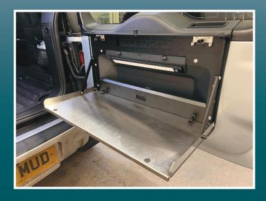
This product can be easily installed with any basic tool kit. There is no need to remove the door-trim from the back door to install the table.
