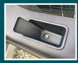
There is an additional hidden fixing within the recessed door-pull. Remove the rubber infill pad from the bottom of the door-pull recess to reveal the hidden screw fixing.
