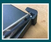
2. The upper corner trims are fixed using 2 x T10 x 8mm and 1 x Tioxizmm fasteners and the M3 nyloc nuts. This is the fiddly part of the table install. Use the T10 screwdriver bit supplied on the fastener heads. If you don't have a spanner to hold the M3 nuts then a pair of needle nose pliers/grips can be used as an effective substitute.
