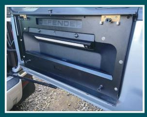
Once all of the fasteners have started in their threads and the spacers sit snug within their recess, tighten all 11 of the fasteners down. With the backplate installed on the door-trim you're now ready to install the fold-down table to the backplate.
