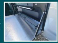
**16.** Use a pair of the thin plastic washers between the table support tabs and the slots in the backplate to prevent metal-to-metal contact as the support tab slides in the channel. Tighten the nyloc nuts on the support tabs just enough that the tabs can still slide freely within the channel on the backplate.
