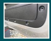
Remove the 11 visible Torx fixings on the rear door-trim using the T30 key supplied. You will not re-use these fasteners for the table install so store them away securely should you wish to remove the table in the future.
