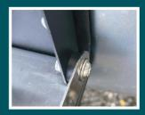
17. Each hinge is made up of 1 x M6x16 Torx fastener, 1 x 6mm spacer block, 1 x Nyloc nut & 1 x M6 washer. The hinge mechanism should be assembled as per the pic. Tighten the nyloc nut just enough so that the table can still rotate freely on its hinge.
