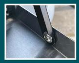
**19.** Push the 6 x nut-caps onto the nuts on the hinge pivots and support tabs.
