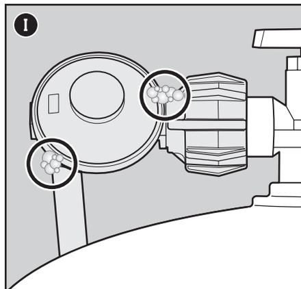
⚠ **DANGER:** Do not use a flame to check for gas leaks. Be sure there are no sparks or open flames in the area while you check for leaks.
