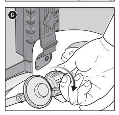
▲ WARNING: The hose must be secured to the tank scale with the Hose Retention Clip. Failure to do so could cause damage to the hose resulting in a fire or explosion which can cause serious bodily injury or death, and damage to property.
