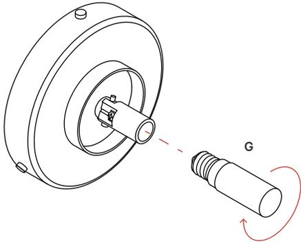
**Step 6:** Align the 15" disc shade (F) with the canopy cover (B) and screw the diffuser into place
