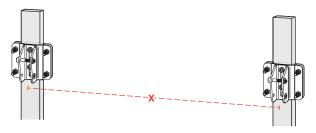
5 Pre-thread two T-slot nuts onto each Awning Mounting Bracket using two M8x14mm bolts, do not tighten.
