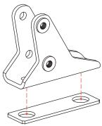
2 Attach one Angle Adjust Bracket to each crossbar using two T-slot nuts and two %" bolts. Place at even positions on the bars. TOOL: 6 mm Hex wrench
