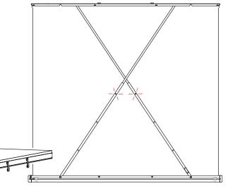
**4** Pull the control lever up to tighten the fabric. You will hear the ratchet mechanism click.
