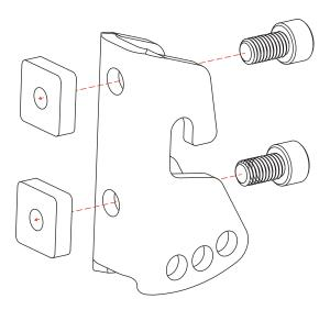
4 Slip the T-slot nuts (with Awning Mounting Bracket in tow) into the T-slots located on the back of the Crosswing Awning using the cutaways at each end.
