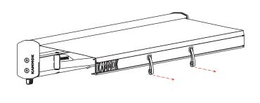
**3** There are three points where the Crosswing will lock into place (located at 3', 4'11", and 6'6"). You will hear two clicks sounding together at each point. These clicks are the spring pins locking the awning into place. The awning cannot be left open at any other location.
