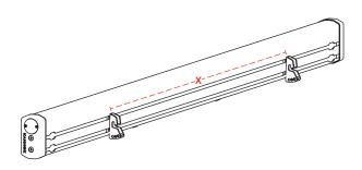
6 With the help of an additional person, lift the Crosswing up to the vehicle. Align the Awning Mounting Brackets with the Angle Adjust Brackets, slot the hook of each Awning Mounting Bracket onto the bolts of the Angle Adjust Brackets, let the Crosswing pivot down until it rests against the Angle Adjust Bracket, the Crosswing will hang safely.
