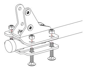
1 Pre-thread one 1 %" bolt with lock washer into the top hole of each Angle Adjust Bracket.
