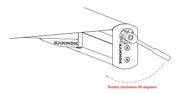
**8** Push inward on the socket so that the tension adjust hex does not push out and lock, allow the socket wrench to slowly spin counterclockwise. (If the tension adjust hex locks and stops turning repeat from step 3 on Page 9 ensuring that you are maintaining inward pressure on the socket).
