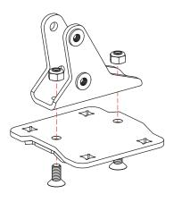
Using additional clamping plate, 4 carriage bolts, and 4 nylon lock nuts, clamp the Angle Adjust Bracket to crossbar. Repeat for other crossbar.
