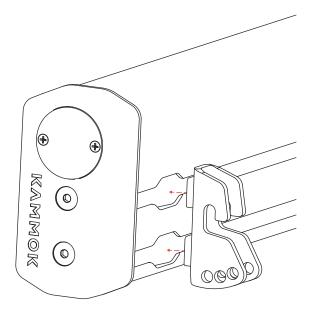
**5** Position the Awning Mounting Brackets to align with the spacing of the Angle Adjust Brackets. Tighten fasteners lightly.
