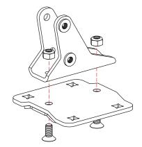
**3** Using additional clamping plate, 4 carriage bolts, and 4 nylon lock nuts, clamp the Angle Adjust Bracket to crossbar. Repeat for other crossbar.
