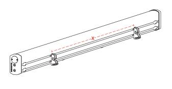
6 With the help of an additional person, lift the Crosswing up to the vehicle. Align the Awning Mounting Brackets with the Angle Adjust Brackets, slot the hook of each Awning Mounting Bracket onto the bolts of the Angle Adjust Brackets, let the Crosswing pivot down until it rests against the Angle Adjust Bracket, the Crosswing will hang safely.
