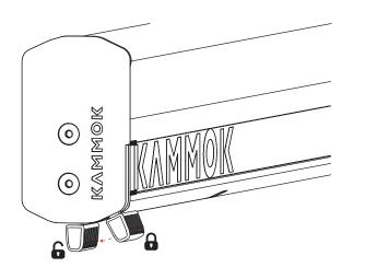
**2** Release Safety strap snaps. Pull the Crosswing open evenly by each safety strap. Do not let go of straps until awning is securely locked in position.
