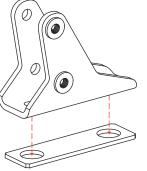
2 Attach one Angle Adjust Bracket to each crossbar using two T-slot nuts and two %" bolts. Place at even positions on the bars. TOOL: 6 mm Hex wrench
