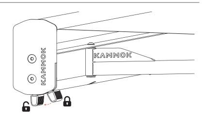
**2** Grab the two safety straps/pull loops. Pull the awning out 2"-3", which will disengage the spring pins.
