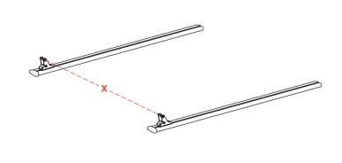
**3** Pre-thread two T-slot nuts onto each Awning Mounting Bracket using two %" bolts, do not tighten.
