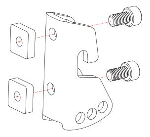
4 Slip the T-slot nuts (with Awning Mounting Bracket in tow) into the T-slots located on the back of the Crosswing Awning using the cutaways at each end.
