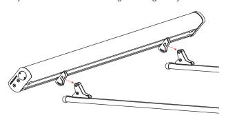
10 Insert one 1 %" into the bottom hole of each Angle Adjust Bracket with the Crosswing lined up at the desired angle. Tighten both 1 %" bolts on each Angle Adjust Bracket.
