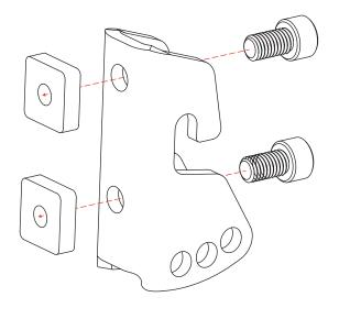
Slip the T-slot nuts (with Awning Mounting Bracket in tow) into the T-slots located on the back of the Crosswing Awning using the cutaways at each end.
