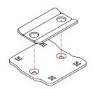
2 Attach one clamping plate to each Angle Adjust Bracket using two flat head bolts and 2 nylon lock nuts.
