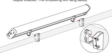
Insert one 1 %" into the bottom hole of each Angle Adjust Bracket with the Crosswing lined up at the Adjust Bracket.
