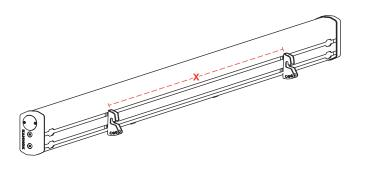
With the help of an additional person, lift the Crosswing up to the vehicle. Align the Awning Mounting Brackets with the Angle Adjust Brackets, slot the hook of each Awning Mounting Bracket onto the bolts of the Angle Adjust Brackets, and let the Crosswing pivot down until it rests against the Angle Adjust
