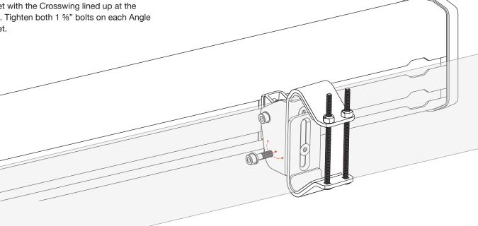
10 If the Crosswing is not at the desired position: slightly loosen the four %" bolts holding the Crosswing to the Awning Mounting Brackets. Slide the Crosswing into the desired position along the length of the vehicle.
