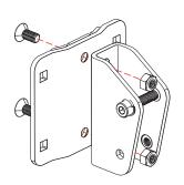
3 Using additional clamping plate, 4 carriage bolts, and 4 nylon lock nuts, clamp the Angle Adjust Bracket to crossbar. Repeat for other crossbar.
