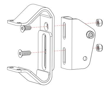
5 Hook the assembly over and around your roof rack bars. Slide the mount assembly into the desired position.
