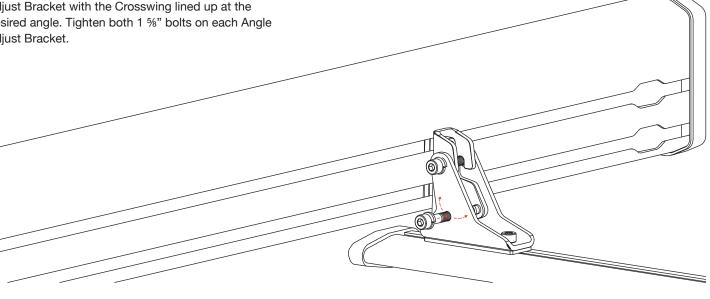
11 If the Crosswing is not at the desired position: slightly loosen the four %" bolts holding the Crosswing to the Awning Mounting Brackets. Slide the Crosswing into the desired position along the length of the vehicle.
