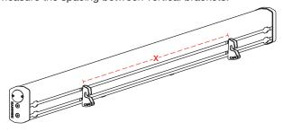
5 Pre-thread two T-slot nuts onto each Awning Mounting Bracket using two 5%" bolts, do not tighten.
