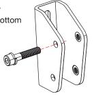
2 Use the awning mountain bolts and a set of Nylock nuts from the stock kit to secure each bracket to the vertical surface.
