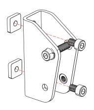
Position the 2 "J" brackets as shown, with the slotted one to the on top/closest to you. Loosely secure the "J" brackets to the vertical brack with 2 flush head bolts and nylock nuts.
