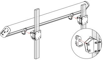
Insert one 1 %" into the bottom hole of each Angle Adjust Bracket with the Crosswing lined up at the desired angle. Tighten both 1 %" bolts on each Angle Adjust Bracket.
