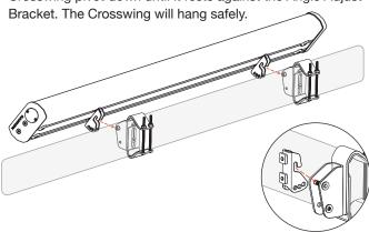
Insert one 1 %" into the bottom hole of each Angle Adjust Bracket with the Crosswing lined up at the desired angle. Tighten both 1 %" bolts on each Angle Adjust Bracket.
