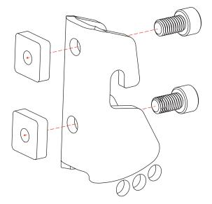
7 Slip the T-slot nuts (with Awning Mounting Bracket in tow) into the T-slots located on the back of the Crosswing Awning using the cutaways at each end.
