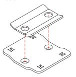
2 Attach one clamping plate to each Angle Adjust Bracket using two flat head bolts and 2 nylon lock nuts.
