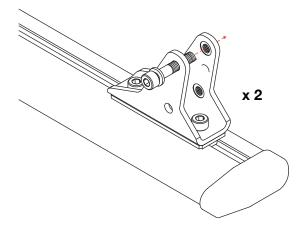
5 Measure spacing between angle adjust brackets.
