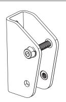
3 Insert the a pivot clamping bolt into the top hole of each bracket. Use an allen wrench to tighten.
