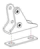
2 Attach one Angle Adjust Bracket to each crossbar using two T-slot nuts and two %" bolts. Place at even positions on the bars.
