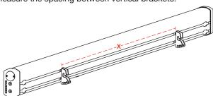
5 Pre-thread two T-slot nuts onto each Awning Mounting Bracket using two %" bolts, do not tighten.
