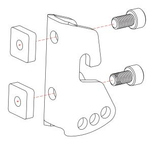
6 Slip the T-slot nuts (with Awning Mounting Bracket in tow) into the T-slots located on the back of the Crosswing Awning using the cutaways at each end.
