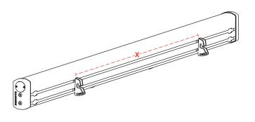
With the help of an additional person, lift the Crosswing up to the vehicle. Align the Awning Mounting Brackets with the Angle Adjust Brackets, slot the hook of each Awning Mounting Bracket onto the bolts of the Angle Adjust Brackets, and let the Crosswing pivot down until it rests against the Angle Adjust Bracket. The Crosswing will hang safely.
