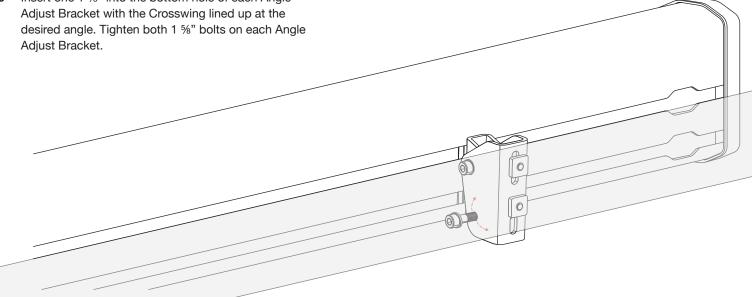
10 If the Crosswing is not at the desired position: slightly loosen the four %" bolts holding the Crosswing to the Awning Mounting Brackets. Slide the Crosswing into the desired position along the length of the vehicle.
