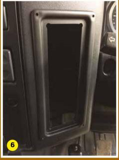
Secure the switch panel in place using the 4 x fixing screws provided. Use a 3mm drill for the fixing holes.
