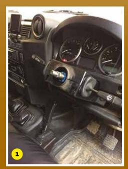
We recommend removing the steering wheel from the vehicle to provide easier access when installing the switch mount.
