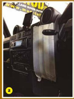
Use masking tape to cover/protect the area that will be cut out of the dashboard.
