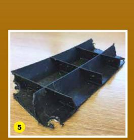
Carefully cut out the section of dashboard. This section of dashboard uses a honeycomb construction. You will need to cut deep enough to fully remove the 15mm depth of the honeycomb webs.
