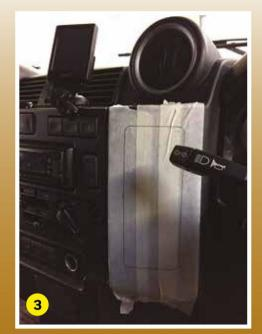
Align the top edge of the cut-out template a minimum distance of 27mm below the top horizontal edge of the dashboard.
