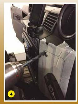
Drill a hole within each corner of the cut-out line large enough to provide access for your saw blade.
