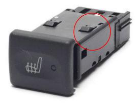
Removing the keyway allows any switch to be fitted into any of the switch holes.
