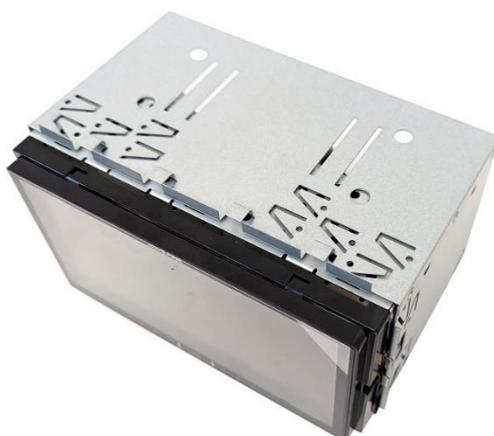
**Step 5-** The trim surround will snap into place and can again be adjusted for preference by going up or down the levels in the fixing peg (make sure you are at the same level, on each of the fixing points).
