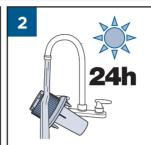
Cyclonic system can be rinsed to clean. Let dry for 24 hours before replacing.
