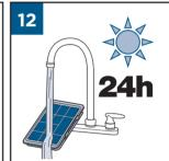
Pleated filter can be rinsed to clean. Let dry for 24 hours before replacing.
