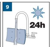
Mesh filter can be rinsed to clean. Let dry for 24 hours before replacing.
