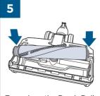
To replace the Brush Roll to the foot, place the left side of the Brush Roll under the belt before pushing down into place.
