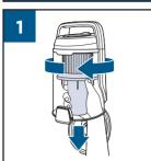
Turn cyclonic system counter-clockwise to release and remove from the tank.
