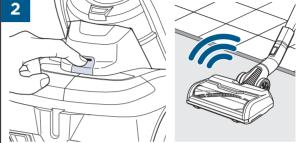
Press Auto Button on back of unit for automatic floor type sensing. The SmartClean canister will detect your floor type and adjust suction as necessary.
