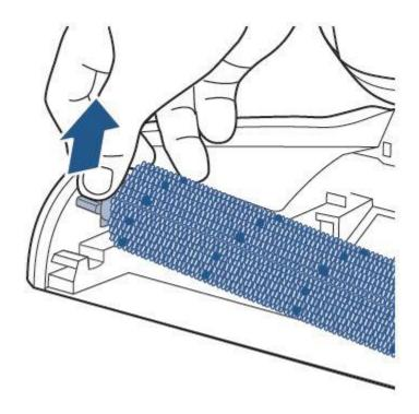
• Clear all debris from brush roll, brush ends, brush gear and brush housing
