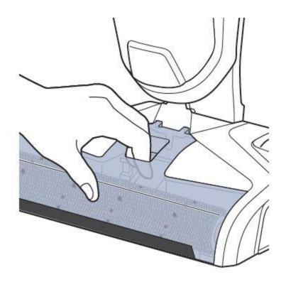
Pull the tab on the left side of the brush roll to remove
