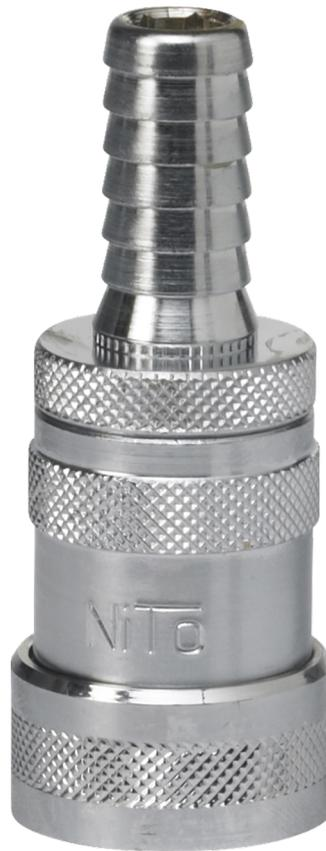
1/2" automatic watertight coupling with water stop when disconnected from quick coupling.
